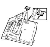
**2** Attach the KX-T7603 to your telephone with screws.
