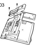
3 Insert the cable into the connector.
